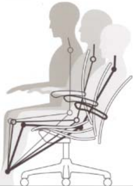
The Kinemat tilt echoes the body's pivot points (ankle, knee, hip) so the Aeron chair moves easily and naturally, shifting weight from the seat to the backrest. The backrest and armrests maintain the same relationship throughout the range of movement, to offer full support in upright or reclined positions.
