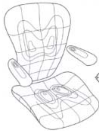
The Pellicle suspension helps to centre weight over the sitting bones and distribute pressure away from the spine and the backs of the thighs, where it can lead to physical problems and discomfort.
